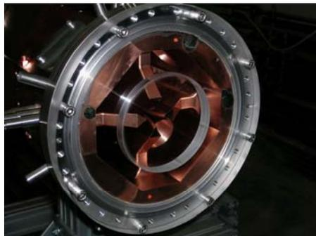
**Fig. 6** Close view of the RFQ accelerating electrodes
