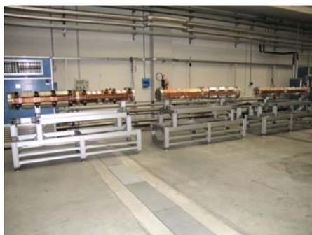
**Fig. 5** The 3 modules of RFQ accelerator ready for RF test
